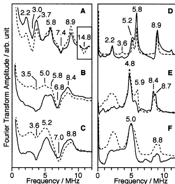
**Figure 1.** Two-pulse (A–C) and three-pulse (D–F) ESEEM spectra of [VO(hybeb)]<sup>2-</sup> recorded at the  $M_I(^{51}\text{V}) = -7/2_{\parallel}$  (A and D),  $-3/2_{\perp}$  (B and E), and  $-1/2_{\perp}$  (C and F) lines. The dashed lines represent simulated spectra. Conditions: frequency, 8.802 GHz; temperature, 13 K; magnetic field, 260.6 (A and D), 304.9 (B and E), 311.3 mT (C and F);  $\tau$  in the three-pulse sequence, 270 (D), 310 (E), 300 ns (F).
